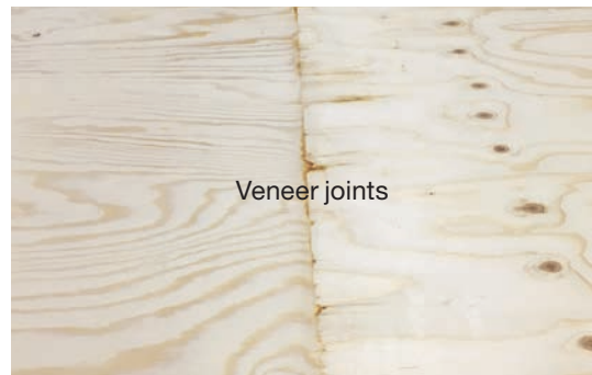
With calibration sanding it is possible that the glue line becomes partially visible.
