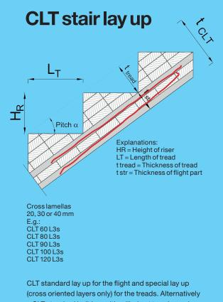
a CLT standard build up with milled out treads can be selected.
