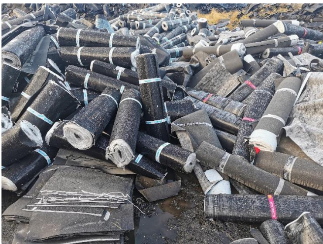
Figure 2 - Roofing felt with defects, delivered as waste directly from manufacturers
