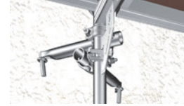
2 wall ties connected in a V-shape with one double coupler each to the inner standard.
