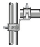
Use of the lattice beam coupler
