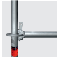
Thanks to the AutoLock-function, the wedge automatically falls into the rosette. The component is secured against shifting and falling out.
